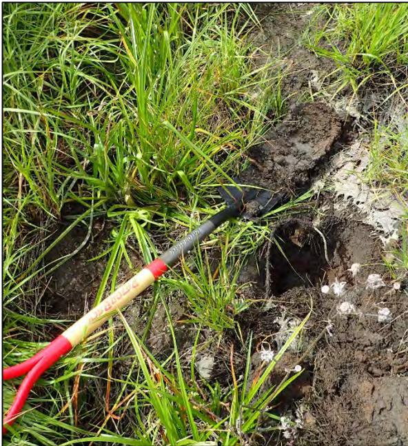
Photograph 2. Close-up view of hydric soils in sample pit SP-01. Meets hydric soils indicator F6, Redox Dark Surface.
