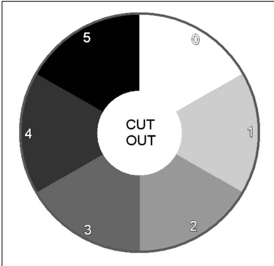
Figure 3-1. Example of a Ringelmann smoker reader chart (Hughes, 2010). The plume is viewed through the cutout and the opacity is compared with the numbered shades on the outer diameters.
