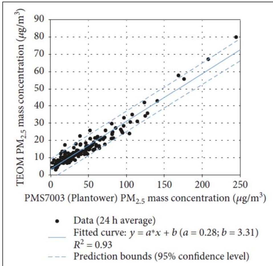
Figure 3-10. Comparison of a Plantower unit (slightly different from but comparable to that used in the PurpleAir) with a TEOM Federal Equivalent Method used for compliance monitoring (Badura et al., 2018). The Plantower is highly correlated, but reads 3.5 times higher than the compliance measurement.
