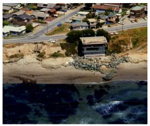
Photo 6-9. Purisima outcrop in front of O'Neill house that serves as a natural groin, which traps littoral drift. (Source: G. Griggs)
