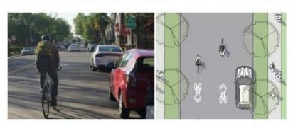
Class IV Separated Bikeway: a bikeway in the roadway separated from vehicle traffic by physical barriers.
