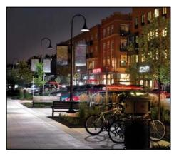
This photo shows pedestrian-scaled lighting which is low enough to the ground to illuminate walkways and the faces of pedestrians.
