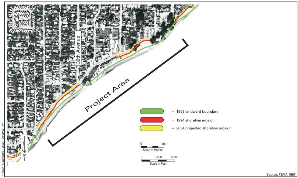
A state-of-the-art soft copy photogrammetry system was used to determine shoreline erosion rates, using aerial photographs spanning 41 years in Santa Cruz County. While some areas of wide sandy beaches have advanced and retreated as a function of storm frequency and nourishment, the bluffs have been eroding at long-term average rates ranging from 6 to 60 centimeters per year.
