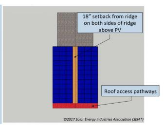
2. For photovoltaic arrays occupying more than 66 percent of the plan view total roof area, not less than a 36-inch (914 mm) clear setback is required on both sides of a horizontal ridge.
